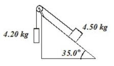
**9.** Two masses are connected by a light string that runs over a frictionless pulley as shown. What is the acceleration of the system when the masses are released and allowed to move?
